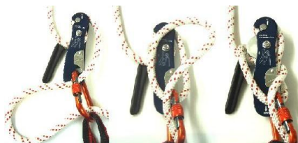
FIGURES 2, 3 AND 4: secure lock-off position
