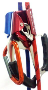
Picture 2: carabiner clipped on blocking cams hole (number 4 of picture 1) prevents the undesired opening of the cams, avoiding accident.
